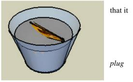
Figure G36: A Coral fragment placed into 30 second RBF cement to create a Coral Plug.
