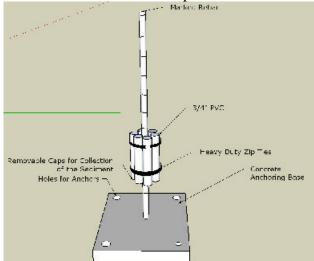
Figure 9: Construction of a basic sediment trap to estimate sedimentation rates at a project site. Sediment accumulates in the PVC tubes, and can be retrieved and measured (by weight or volume) by removing the caps at the bottom of the PVC tubes and collecting the sediment within. <u>Note:</u> This method only provides a relative estimate of the amount of sediment at a specific depth, and not an exact value because it measures the vertical settling of sediment, and not horizontal transport.
