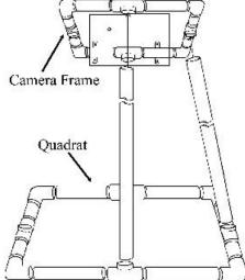
Figure G30: Camera monitoring frame or quadrat framer. This device is built so that most standard underwater digital cameras can screw into the plate in the center of the camera frame, and will take a picture downwards towards the quadrat. The quadrat allows the photo to be standardized for length.
