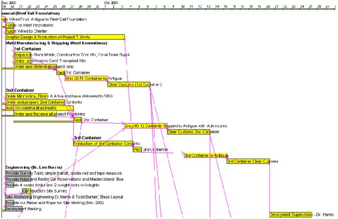
Figure 3b: Portion of a complex Gantt chart generated by PlanBee software to aid in the project management of the deployment of over 3,500 reef modules and planting of 10,000 coral fragments and 14 tons of adult coral transplants in Antigua, 2003-2004.
