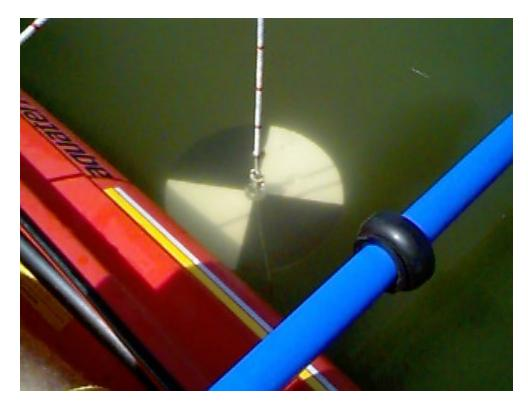
Markings or knots on the rope identify the distance of the disk from the water surface. The disk is lowered into the water until it disappears and the depth recorded, then the disk is raised until it reappears and the depth recorded. The two depths are averaged and this becomes the Secchi visibility. Usually, the color of the water is also noted.
