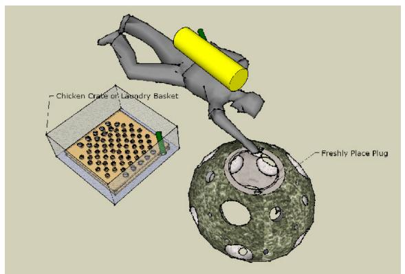
Figure G34: Schematic of diver planting coral plugs from a Coral Planting Tray onto a Reef Ball. The diver can use the tray to store supplies such as a wire brush, or extra epoxy putty. Planting teams need to be trained on the project's planting strategy to know where to plant coral plugs
