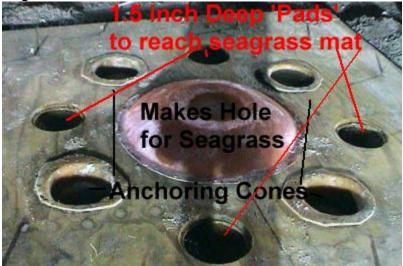
Figure 22: An advanced anchoring technique adapted for use in a sea grass bed. This technique produces cone anchors (Figure 20), but is adapted to allow the sea grass under the Reef Ball to stay alive.
