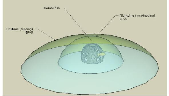
Figure 4: Illustration of effective protective void space (EPVS) for Damselfish on a Pallet Ball sized Reef Ball categorized by daytime and nighttime foray. For example, nighttime EPVS for the abovepictured Damselfish in a Pallet Ball would be approximately 16.5 cubic meters (592 cubic feet) if one based the radius of the foray (sphere shaped) around the reef module at 2 meters (6 feet 7 inches).
