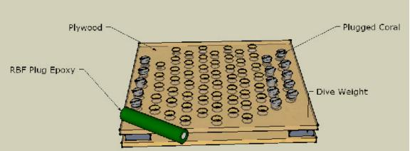
Figure G18: Diagram of Coral Curing and Planting Tray (available in Sketch Up  $^{TM}$ ). Coral Plugs fit into the holes drilled in the top board, which can be made from plywood or, if available, more water resistant materials such as resin or plastic.
