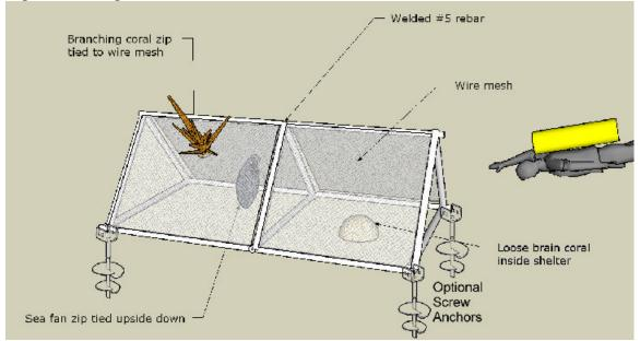
Figure 2: A temporary disaster nursery constructed from wire mesh attached to a tetrahedral frame made from welded steel. Imperiled corals would be attached to the wire mesh with plastic cable ties or thin wire to protect them from damage by waves or sedimentation until a permanent solution can be implemented. If necessary, "disaster nurseries" can be anchored with screw anchors
