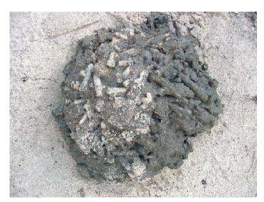
Figure 13: Reef Forms are large blobs of concrete cast into a mold made of sand and affixed with coral adapter plugs. Reef Forms
