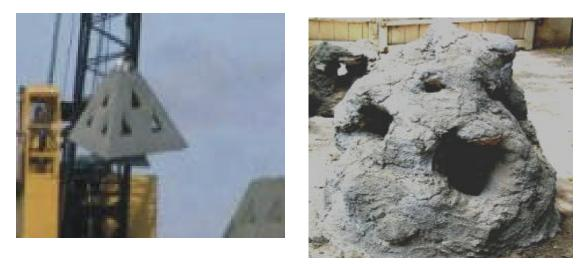
Figure 16: Concrete modules designed primarily for 'fish only' projects. Left: Artificial Reefs 1 Fish Haven  $\mathbb{M}$  Modules. Right: Hand made 'Fish Houses'. Modules of these types are not recommended for coral rehabilitation techniques discussed in this manual because they utilize support frames made from metal, which can reduce the long term durability and stability of the module.
