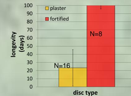
Figure 9: Mean longevity of PoP discs vs. discs fortified with 10% sand and 10% portland cement. 6 of 8 fortified discs are still intact after 120 days.
