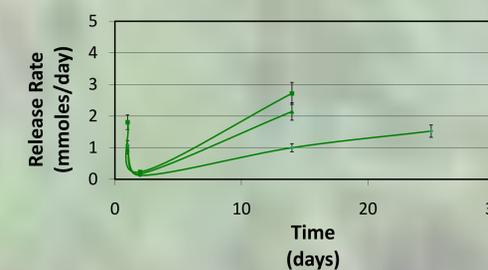
Figures 3 & 4: Release rate in millimoles of N (left) and P (right) per day for three identical replicated PoP discs with 50 grams of fertilizer each. Two of the discs were destroyed after 15 days, the third lasted 25 days
