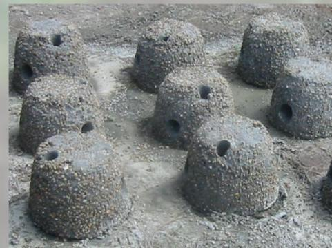
Figure 2: Armored cultivator units post production awaiting deployment. (photo: J. Krumholz)
