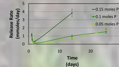
Figures 5 & 6: Release rate in millimoles of N (left) and P (right) per day for three PoP discs with varying fertilizer concentrations. Molar addition calculations are based on conversion from percent by volume. One of the discs were destroyed after only 15 days, the other two lasted 25 days
