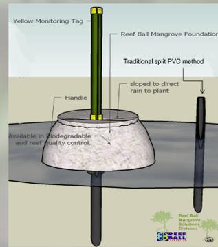
Figure 1: Conceptual drawing of armored cultivator mangrove rehabilitation unit. (image courtesy of www.mangrovesolutions.com)
